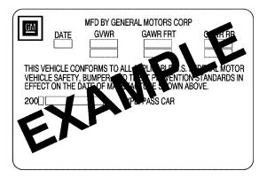
A vehicle specific Certification label is attached to either the driver's door edge or the lower center pillar on the driver's side of the vehicle. This label shows the gross weight capacity of your vehicle, called the Gross Vehicle Weight Rating (GVWR). The GVWR includes the weight of the vehicle, all occupants, fuel, and cargo.
